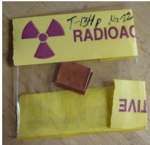
Figure 34. Picture of the copper standard source used to calculate the 3\gamma/2\gamma correction factor.
