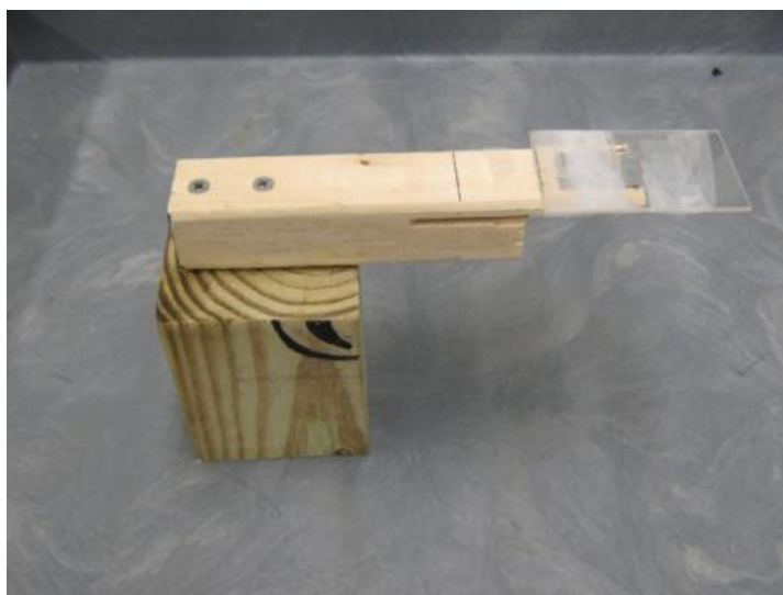
Figure 16. Holder developed by 2 nd Lt Robert Slaughter to allow calibration sources to be centered inside the detector.
